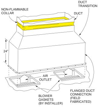
FIGURE 13 - SUGGESTED METHOD FOR CONNECTING DUCTWORK
